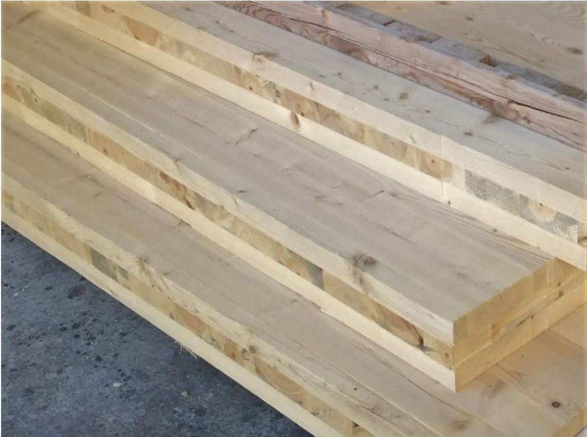
*Image 3: Cross Laminated Timber (CLT).*
